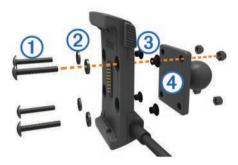
2 Tighten the nuts to secure the base plate.
