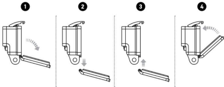
1. Open the Backdoor of the housing so that it is hanging downwards.
