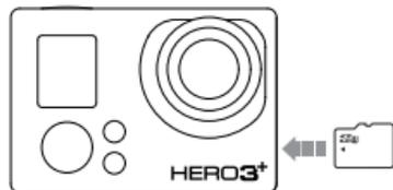
1. Slide memory card into card slot with label facing front of camera.
