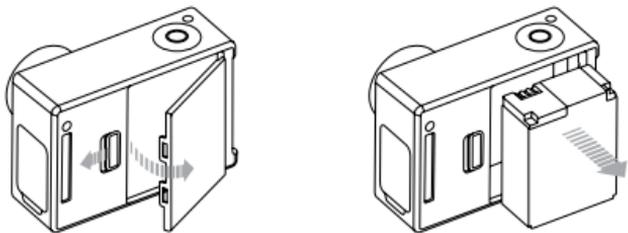
1. Remove the battery door by placing your thumb in the indentation in the battery door (on the back of the camera) and sliding it to the left.
